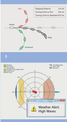
The ASM collects data from navigational, meteorological and safety sensors. It then assesses this data to build a local map of objects and potential hazards. This approach fuses and correlates data from multiple sensors to reduce overall uncertainty and improve the quality and integrity of the so-called world perception model. This overall perception is used as a basis to determine appropriate actions under the prevailing conditions.
