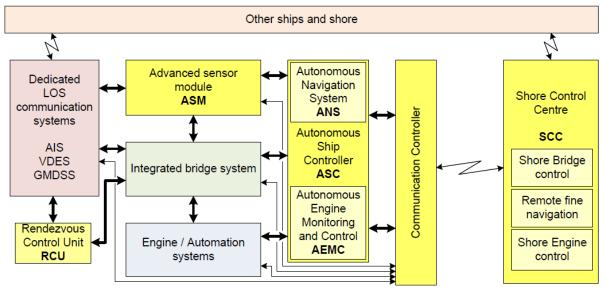
Figure 1: Overview of high level modules /8/
