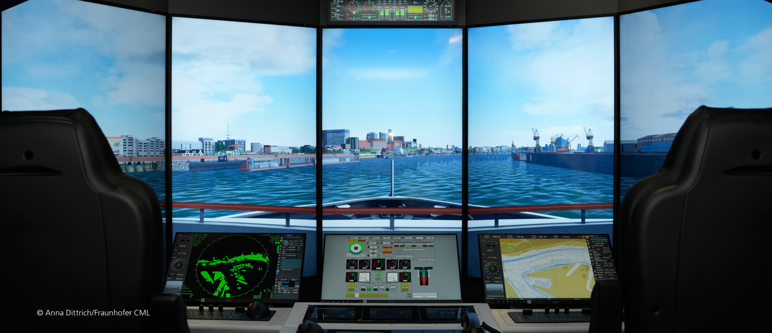
Ship simulators are used at the Fraunhofer CML to test autonomous technologies
